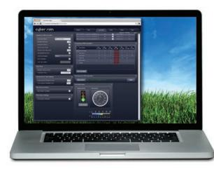
Cyber Rain's irrigation tool (above) uses weather predictions retrieved through the Internet to automatically manage watering schedules for landscaped properties. The result is huge water savings.
